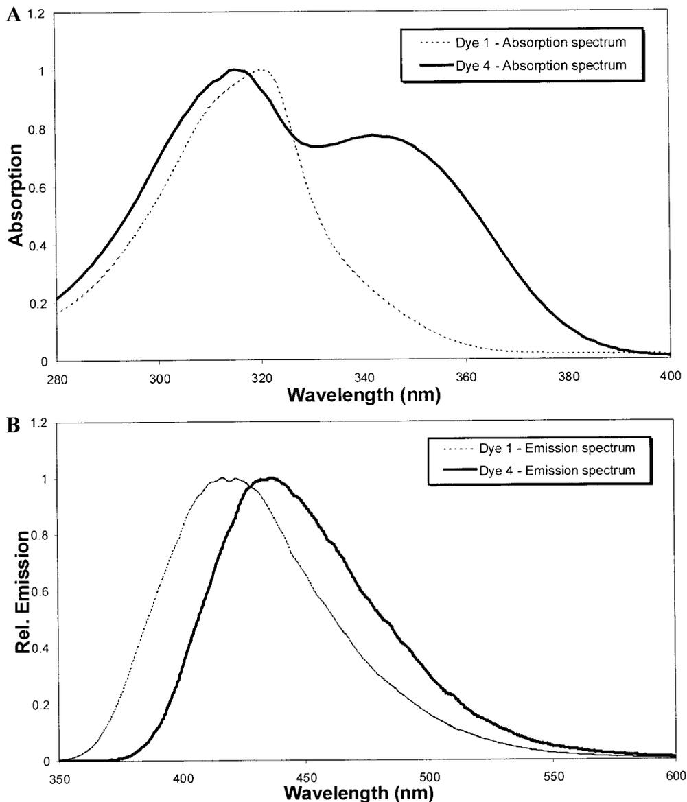
**FIG. 3.** (A) Absorption and (B) emission spectra of dyes 1 and 4 ( $\text{H}_2\text{O}$ , pH 7,  $20^\circ\text{C}$ ). The excitation wavelengths for dyes 1 and 4 were 320 and 317 nm, respectively.
