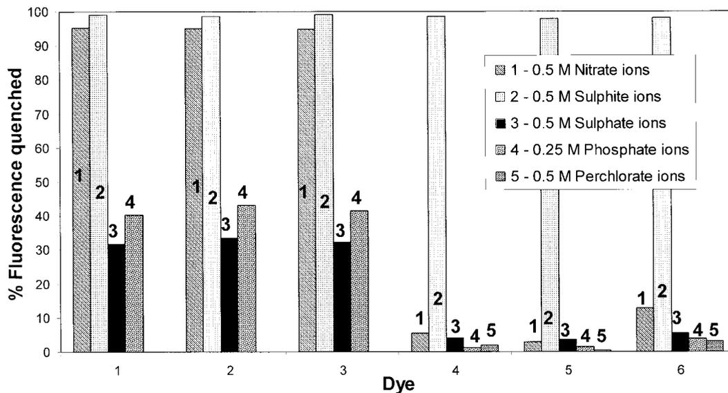
FIG. 5. Percentage fluorescence quenched of  $10^{-6}$  mol dm $^{-3}$  dye 1–6 solutions by various aqueous anions. Dyes 1–3 were not quenched by perchlorate ions.
