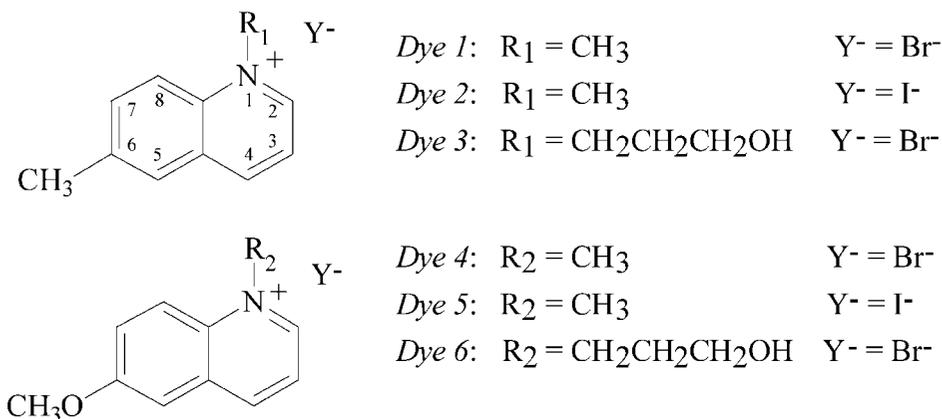
**FIG. 1.** Fluorescent dyes 1–6 and the numbering system of quinoline. The synthesis of dyes 4–6 has been described by the authors previously (9).
