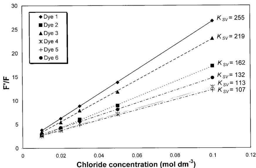
FIG. 4. Stern–Volmer plots for dyes 1–6 quenched by chloride ions,  $\text{H}_2\text{O}$ , pH 7,  $20^\circ\text{C}$ .  $K_{SV}$  units,  $\text{mol}^{-1} \text{dm}^3$ .
