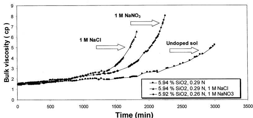
**Figure 10.** The effect on the bulk viscosity and hence  $t_g$  by adding inorganic salts. 1 M NaNO<sub>3</sub> and 1 M NaCl sols were prepared by adding 4.25 g and 2.92 g of the respective salts to 50 ml of sol containing 10<sup>-5</sup> M JA120. Bulk viscosities were recorded using Ostwald viscometers.
