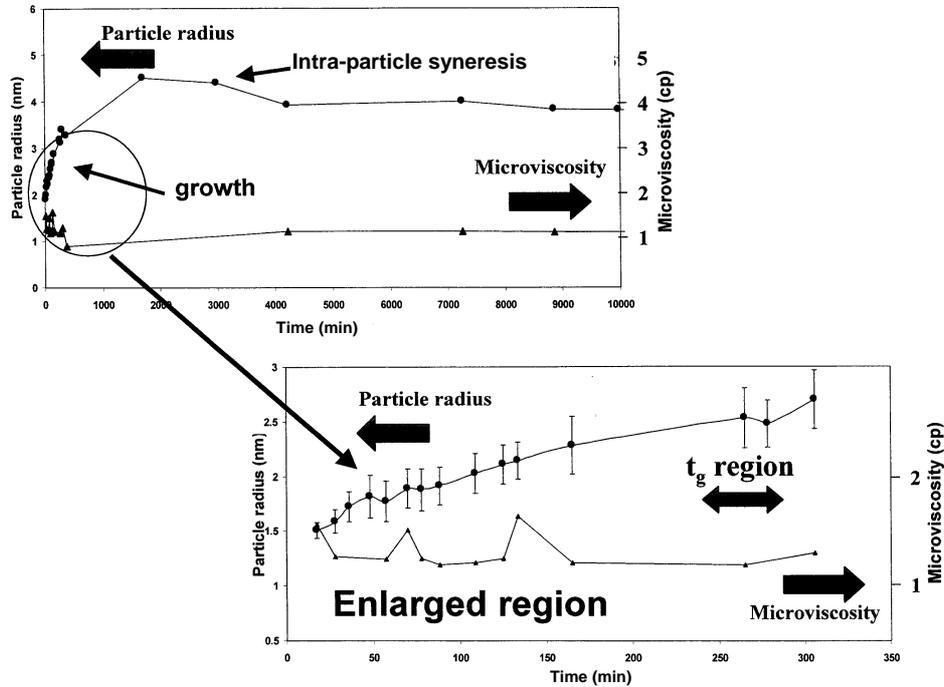
**Figure 5.** Typical silica particle radii and sol microviscosity across the sol-to-gel transition at  $t_g$ , for a 12.70% SiO<sub>2</sub> (final w/w) sol-gel, with an excess acid pH of 0.9. For this data the growth rate constant  $k = 8.6 \cdot 10^{-5} \text{ s}^{-1}$ .
