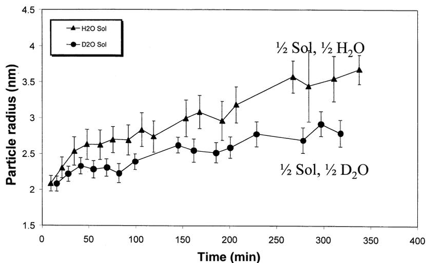
**Figure 7.** Silica particle growth in the absence and presence of  $\text{D}_2\text{O}$ . Errors in silica particle radii were calculated from three times the standard deviation of the bound dye rotational correlation time,  $\tau_{r2}$ .
