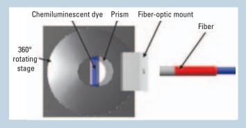
Top view of the experimental geometry and major components used for SPCC.
