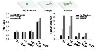
*Figure 2.* Triangle and bow-tie 2.5 mm equilateral structures 50 nm thick were vapor deposited on Ag continuous films 40 nm thick and glass slides (BOT, signal detection at bottom; TOP signal detection at top). Polarization ratios for MT-SPCC sample geometries (left). Intensity enhancement factor (Mw/no Mw) for MT-SPCC sample geometries (right).
