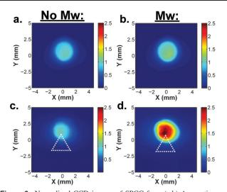
*Figure 3.* Normalized CCD images of SPCC from (a,b) Ag continuous films 40 nm thick and (c,d) Ag continuous films 40 nm thick modified with 2.5 mm Ag triangle structures 50 nm thick, before (no Mw) and during (Mw) application of a short microwave pulse.
