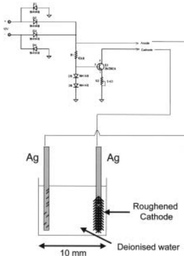
Fig. 2. Constant current circuit apparatus for silver fractal growth.
