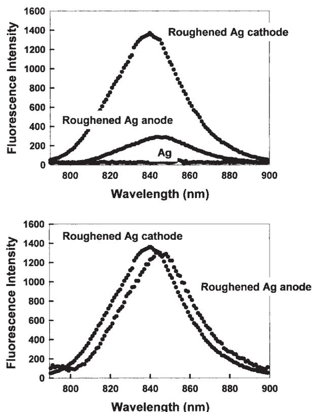
**Fig. 6.** Top, Fluorescence intensity of HSA-ICG-coated roughened silver electrodes and an unused silver electrode, Ag;  $\text{Ex} = 760 \text{ nm}$ . Bottom, Fluorescence intensities normalized to the intensity of the ICG-HSA-coated silver cathode. It should be noted that the normal fluorescence emission maximum ( $\text{H}_2\text{O}$ , pH 7) of 810 nm is shifted in this regard because of the choice of filters that were required to discriminate against a highly scattering silver surface.
