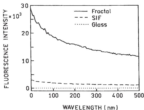
Fig. 11. Photostability of FITC-HSA deposited on glass (.....), a silver island film (-----), and fractal silver structures on SnCl<sub>2</sub>-treated glass (—). The samples were excited at 514 nm.
