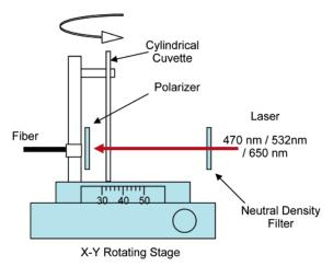
**Figure 1.** Coordinate system used to describe the geometrical arrangement of the illumination (Perp. excitation) and detection systems (top) and the apparatus used for measuring the angular dependence of colloidal scatter (bottom).
