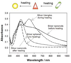
**Figure 4.** Absorption spectra of silver spheres and silver nanorods before, during, and after heating at 40 °C in solution.
