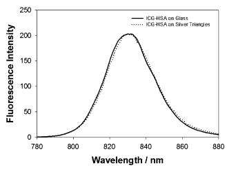
**Figure 5.** (Top panel) Fluorescence emission intensity of ICG-HSA on silver triangles with different loading densities. The emission intensity of ICG-HSA is 75. (Bottom panel) Normalized emission intensities of ICG-HSA and glass and on silver triangles ( $A_{550} = 0.03$ ), which shows identical spectral behavior.
