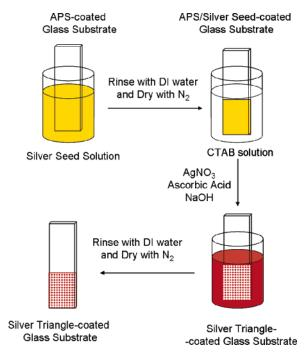
Figure 1. Deposition of silver triangles onto glass substrates.
