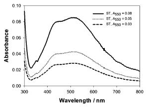
Figure 2. Absorption spectra of silver triangles deposited on glass substrates.
