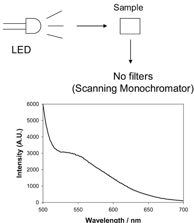
**Figure 1.** Experimental setup for wavelength-dependent ratiometric-scattering based glucose sensing (top) and wavelength-dependent scattering from LUDOX (30 nm) particles upon white LED illumination (bottom).
