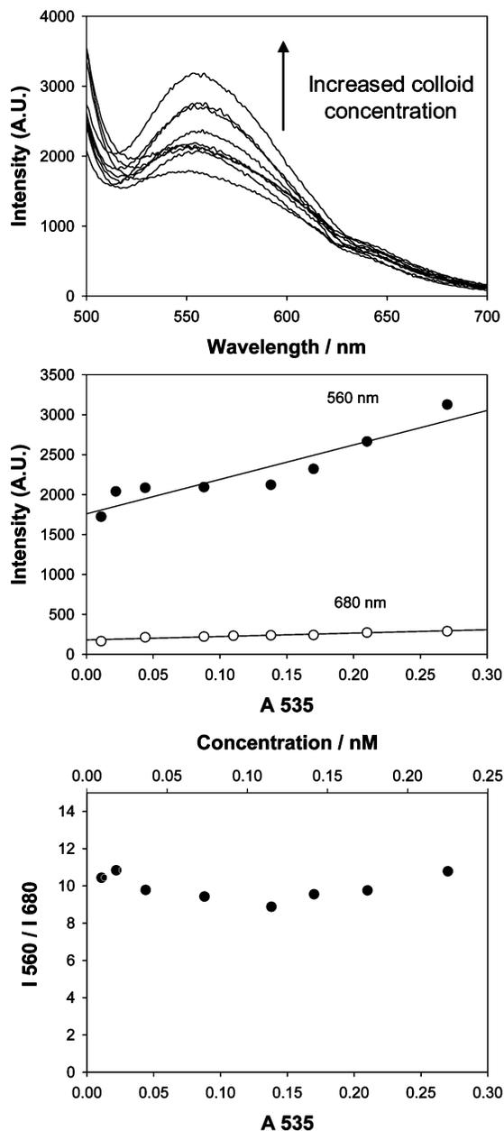
**Figure 3.** Wavelength-dependent scattering from dextran-coated gold nanoparticles upon white LED illumination (top), scattered intensities at 560 and 680 nm vs concentration of the same nanoparticles (middle), and ratios of the scattered intensities vs concentration of the same nanoparticles (bottom).
