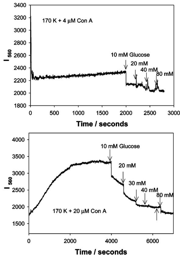
**Figure 6.** Time-dependent scattering intensity of dextran-coated gold nanoparticles in the presence of glucose and 4 (top) and 20  $\mu\text{M}$  Con A (bottom) upon white LED illumination.
