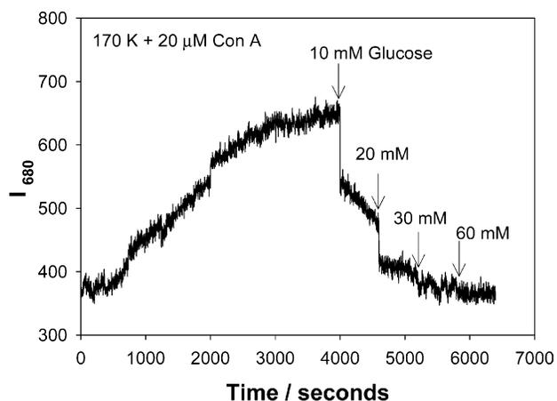
**Figure 8.** Time-dependent scattering intensity measured at 680 nm for 170k dextran-coated gold nanoparticles in the presence of glucose and 20  $\mu\text{M}$  Con A, upon white LED illumination.
