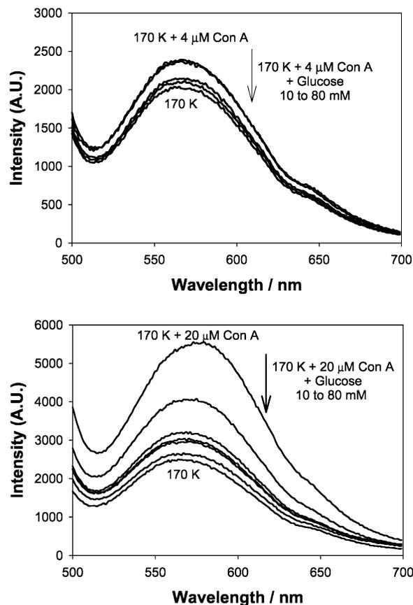
**Figure 4.** Wavelength-dependent scattering from dextran-coated gold nanoparticles after the addition of glucose with 4 (top) and 20  $\mu$ M Con A (bottom) upon white LED illumination.
