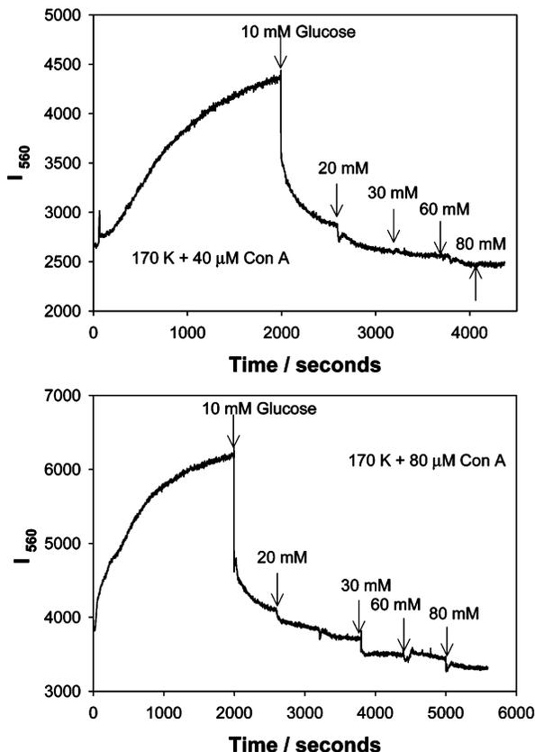
**Figure 7.** Time-dependent scattering intensity of dextran-coated gold nanoparticles in the presence of glucose and 40 (top) and 80  $\mu\text{M}$  Con A (bottom) upon white LED illumination.
