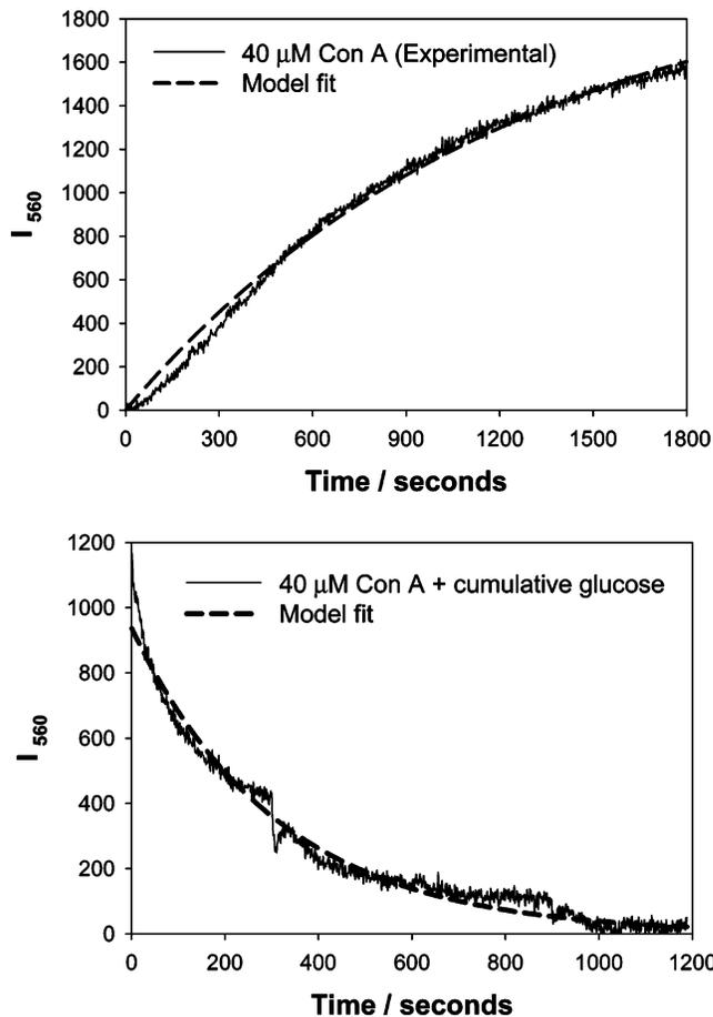
**Figure 9.** Fitting of eq 1 to the 560-nm time-dependent scattering for 40  $\mu\text{M}$  Con A induced nanogold aggregation (top), and eq 3 to the dissociation of the same sensing aggregate by glucose (bottom).
