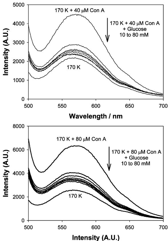
**Figure 5.** Wavelength-dependent scattering from dextran-coated gold nanoparticles after the addition of glucose with 40 (top) and 80  $\mu\text{M}$  Con A (bottom) upon white LED illumination.
