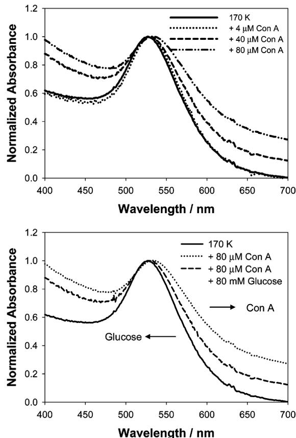
**Figure 2.** Normalized absorbance spectra of dextran-coated gold nanoparticles in the absence and in the presence of Con A (top) and after the addition of glucose (bottom). The absorbance of dextran-coated gold nanoparticles at 535 nm was 0.20 (0.16 nM; this concentration was used for the remainder of the paper).
