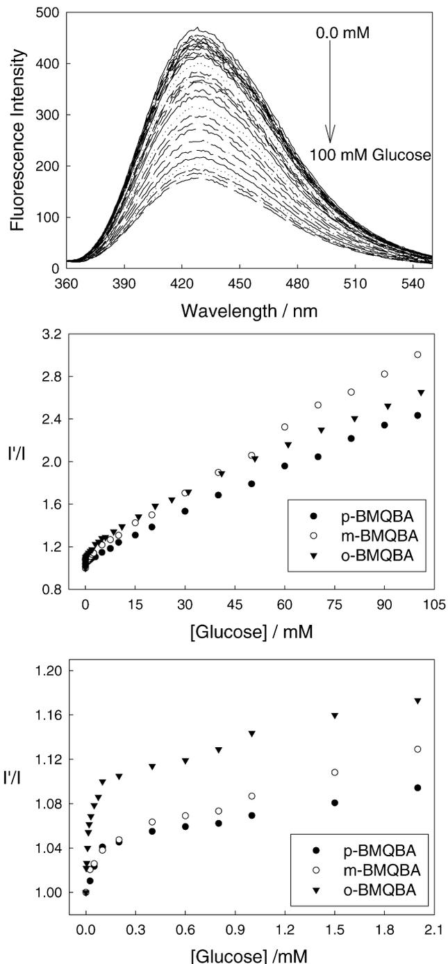
Fig. 5. Emission spectra of *o*-BMQBA in pH 7.5 phosphate buffer with increasing glucose concentrations (top), the respective 427 nm intensity ratio for all three isomers in the absence  $I'$ , and presence  $I$ , of glucose, respectively (middle) and in the low concentration range of glucose, shown to correlate with tear glucose levels (bottom).
