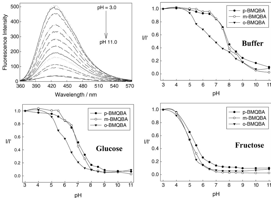
**Fig. 3.** Fluorescence spectra of *o*-BMQBA in buffer media (top left).  $\lambda_{ex} = 320$  nm. Emission intensity at 427 nm  $I$ , divided by the initial emission intensity,  $I'$ , as a function of pH (top right) and with 100 mM glucose (bottom left) and 100 mM fructose (bottom right).
