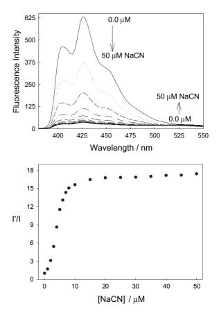
Fig. 5. Fluorescence emission spectra of ANDBA with increasing concentrations of aqueous cyanide (top) and the respective ratiometric type plot using the initial fluorescence intensity, I', at 425 nm in the absence of cyanide, and in the presence of increasing cyanide concentrations, I (bottom).
