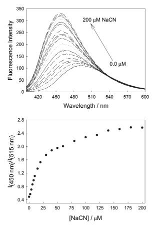
Fig. 2. Fluorescence emission spectra of DSTBA with increasing concentrations of aqueous cyanide (top) and the respective ratiometric plot using the intensities at 450 and 515 nm (bottom).
