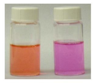
Fig. 7. Photograph of two vials containing equal concentrations of PANSBA with both 0 and 50  $\mu$ M NaCN (left and right, respectively).
