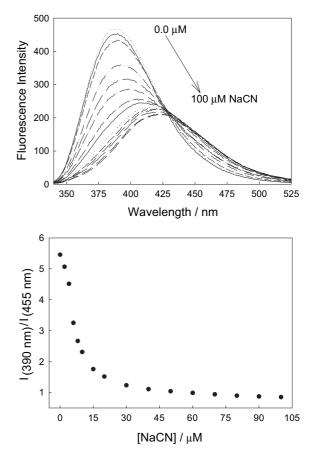
Fig. 3. Fluorescence emission spectra of CSTBA with increasing concentrations of aqueous cyanide (top), and the respective ratiometric plot using the intensities at 390 and 455 nm (bottom).
