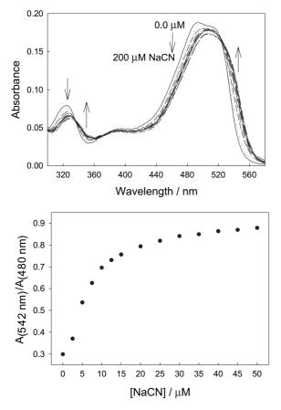
Fig. 6. Absorption spectra of PANSBA with increasing concentrations of aqueous cyanide (top) and the respective ratiometric plot using the intensities at 542 and 480 nm (bottom).
