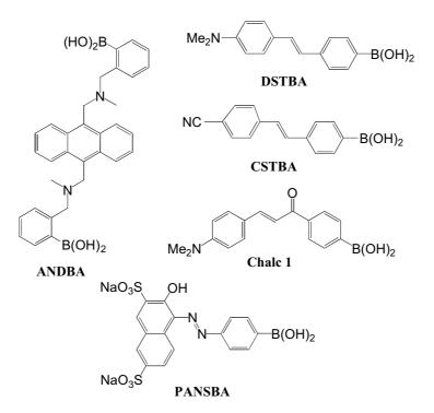
Fig. 1. Molecular structures of probes screened for their interactions with aqueous cyanide. DSTBA, 4'-dimethylaminostilbene-4-boronic acid; CSTBA, 4'-cyanostilbene-4-boronic acid; Chalc 1, 3-[4'(dimethylamino)phenyl]-1-(4'-boronophenyl)-prop-2-en-1-one; ANDBA, 9,10-bis[[*N*-methyl-*N*-(*o*-boronobenzyl)amino]methyl]-anthracene; PANSBA, 1-(4-boronophenylazo)-2-hydroxy-3,6-naphthalenedisulfonic acid disodium salt.
