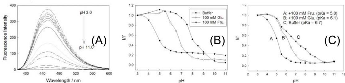
Fig. 6- Emission spectra of *o*-BMOQBA in buffer media (A),  $\lambda_{ex} = 345$  nm. Emission intensity at band maximum,  $I$ , divided by the initial intensity,  $I'$ , for *o*-BMOQBA (B), and *o*-BMQBA (C).
