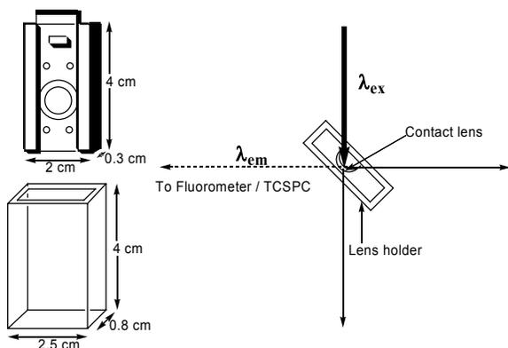
Fig. 2. Contact lens mount and quartz holder (left). The experimental geometry used in the sensing study using lens (right).
