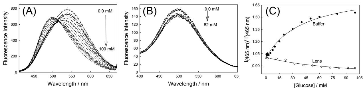
Fig. 4- Emission spectra of DDPBBA in pH 8.0 phosphate buffer-methanol (2:1) with glucose (A), in lens (B),  $\lambda_{\text{ex}} = 340$  nm. Ratiometric response of the probe in buffer and lens with glucose (C).
