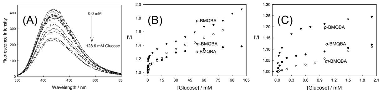
Fig.10- Emission spectra of *o*-BMQBA in contact lens with glucose (A),  $\lambda_{ex} = 320$  nm. The respective 427 nm intensity ratio in the absence,  $I'$ , and in the presence of glucose,  $I$ , for all three isomers (B), and in the low concentration range of the glucose (C).
