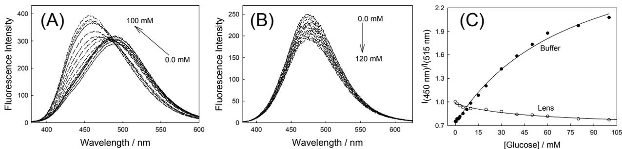
Fig. 3- Emission spectra of DSTBA in pH 8.0 phosphate buffer-methanol (2:1) with glucose (A), in lens (B),  $\lambda_{\text{ex}} = 340$  nm. Ratiometric response of the probe in buffer and lens with glucose (C).
