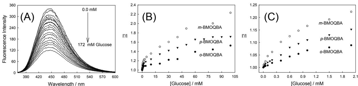
Fig. 8- Emission spectra of *o*-BMOQBA in contact lens with glucose (A),  $\lambda_{\text{ex}} = 345$  nm. The respective 450 nm intensity ratio in the absence,  $I'$ , and in the presence of glucose,  $I$ , for all three isomers (B), and in the low concentration range of the glucose (C).
