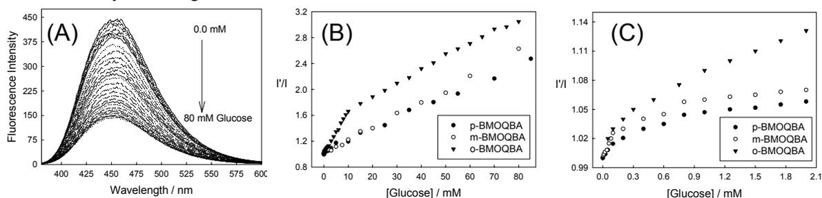
Fig. 7- Emission spectra of *o*-BMOQBA in pH 7.5 phosphate buffer with glucose (A),  $\lambda_{\text{ex}} = 345$  nm. The respective 450 nm intensity ratio in the absence,  $I'$ , and in the presence of glucose,  $I$ , for all three isomers (B), and in the low concentration range of the glucose (C).
