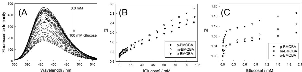
Fig. 9- Emission spectra of *o*-BMQBA in pH 7.5 phosphate buffer with glucose (A),  $\lambda_{ex} = 320$  nm. The respective 427 nm intensity ratio in the absence,  $I'$ , and in the presence of glucose,  $I$ , for all three isomers (B), and in the low concentration range of the glucose (C).
