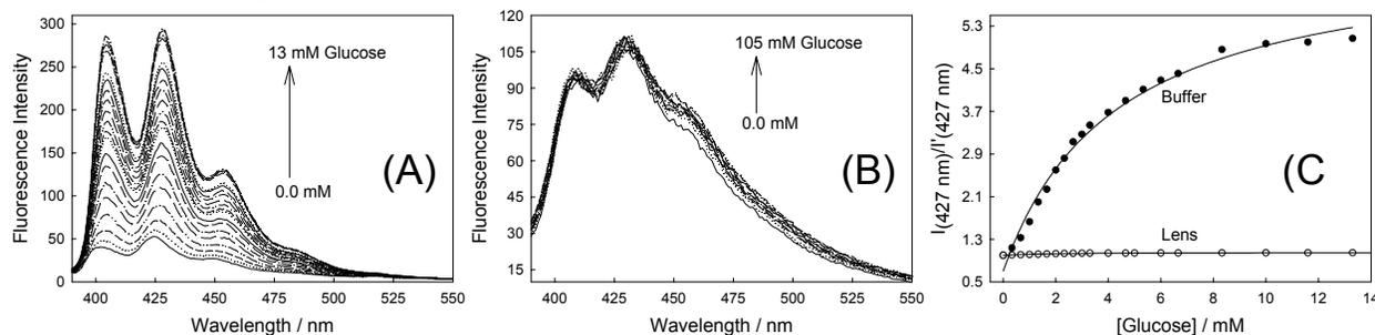
Fig. 5- Emission spectra of ANDBA in pH 8.0 buffer-methanol (2:1) with increasing concentrations of glucose (A), in lens (B),  $\lambda_{\text{ex}} = 340$  nm, and response with glucose in buffer and lens (C).
