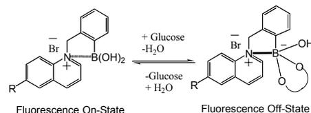
Scheme 1- A schematic representation of the sensing mechanism for the charge neutralization mechanism.
