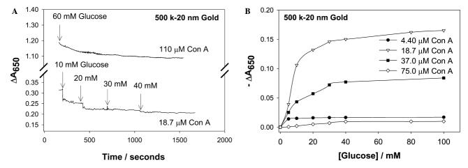
Fig. 10. Time-dependent cumulative change in absorbance at 650 nm for 500 k dextran-coated gold nanoparticles after the addition of glucose (A), Cumulative change in absorbance at 650 nm for 500 k dextran-coated gold nanoparticles versus the concentration of glucose (B).
