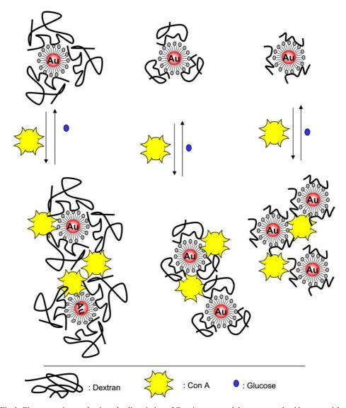
Fig. 1. Glucose sensing mechanism: the dissociation of Con A-aggregated dextran-coated gold nanoparticles.
