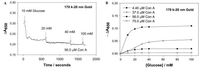
Fig. 11. Time-dependent cumulative change in absorbance at 650 nm for 170 k dextran-coated gold nanoparticles after the addition of glucose (A), Cumulative change in absorbance 650 nm for 170 k dextran-coated gold nanoparticles versus the concentration of glucose (B).
