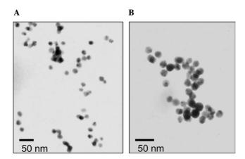
Fig. 9. TEM images of 170 k dextran-coated 20-nm gold nanoparticles before (A) and after (B) the addition of 110 mM Con A.
