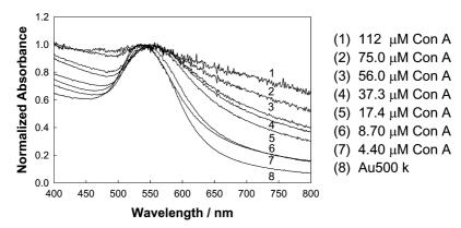
Fig. 5. Normalized absorption spectra of 500 k dextran-coated 20-nm nanogold, cross-linked with different concentrations of Con A.
