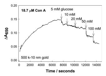
Fig. 13. Time-dependent change in absorbance at 650 nm for 500 k dextran-coated 10-nm gold nanoparticles and the subsequent reduction in  $\Delta A_{650}$  by the addition of glucose, i.e.,  $-\Delta A_{650}$ .
