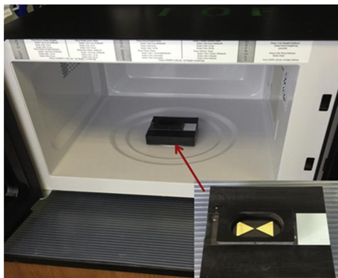
**Fig. 2.** Household microwave fitted with a mounting device designed to hold the lysing chamber as shown in the inset.
