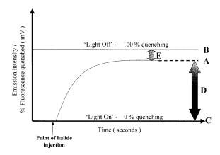
**Figure 3.** A typical oscilloscope display. The millivoltmeter is used in conjunction with the oscilloscope at high degrees of fluorescence quenching to obtain accurate values. A, The light intensity (mV) in the presence of halide ions; B, 'light off', the position of 100% fluorescence quenching; C, 'light on', the position when no halide is present; D, the quenched emission intensity (mV); and E, the final observed emission intensity (mV).
