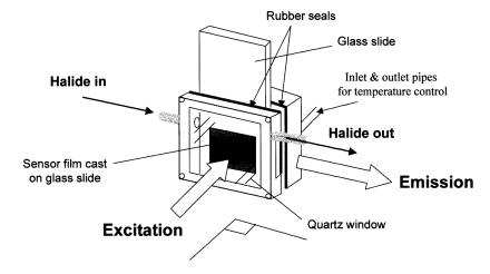
Figure 1. The optical flow cell.
