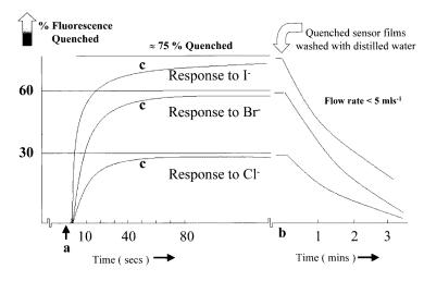
**Figure 4.** The sensor-film response to 1 M halide solutions. The same film is used for all three response curves. Washing quenched films with distilled water returns the films to their original fluorescence intensity. a, The point of halide injection at time t = 0; b, the point of injection of distilled water into the flow cell; and c, the roughly 90% sensor-response point.
